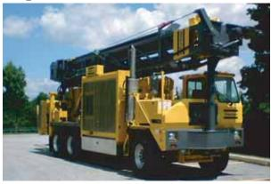
With the addition of a new design Atlas Copco T4W Rig to our existing fleet of modern drilling equipment. B. L. Myers Bros has once again taken steps to improve quality & performance with its features like 1070/350 air supply, 50,000 pound pull back, 25' drill rods, spur gear rotary head and 600 horsepower QSX15C Cummings tier 111 emission complaint engine. This gives the rig the power to drill 20 inch holes at depths of 2,000 feet quickly and efficiently.
